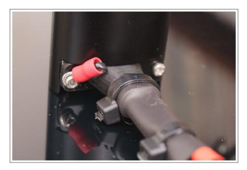
**For 'long can' base with connector facing down:** Re-assemble the 2 long screws, the screws do throw the holes of the kit's base joint, take care that the red ground hook is attached to one of the screws, and then replace the 2 screws sleeves. Fix the screw to tonearm's base and slid back the can into the original position.
