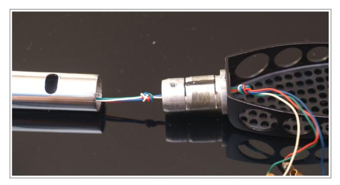
4) Gently remove the wire pulling them out from the arm tube. Take cares that the black wire is not disturbed in the operation
