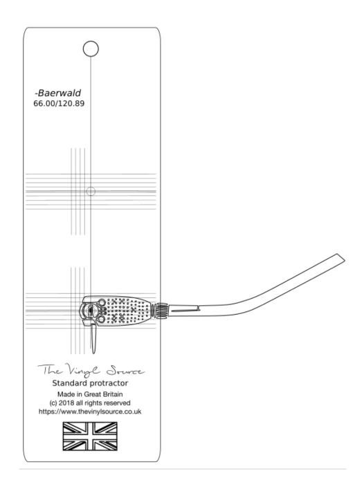
You will probably need to make some adjustment in the cartridge position, if you did so check again the position described in step 2, and, eventually, recorrect. You might need to repeat the steps 2 and 3 few times until the cartridge is aligned with either grids.
