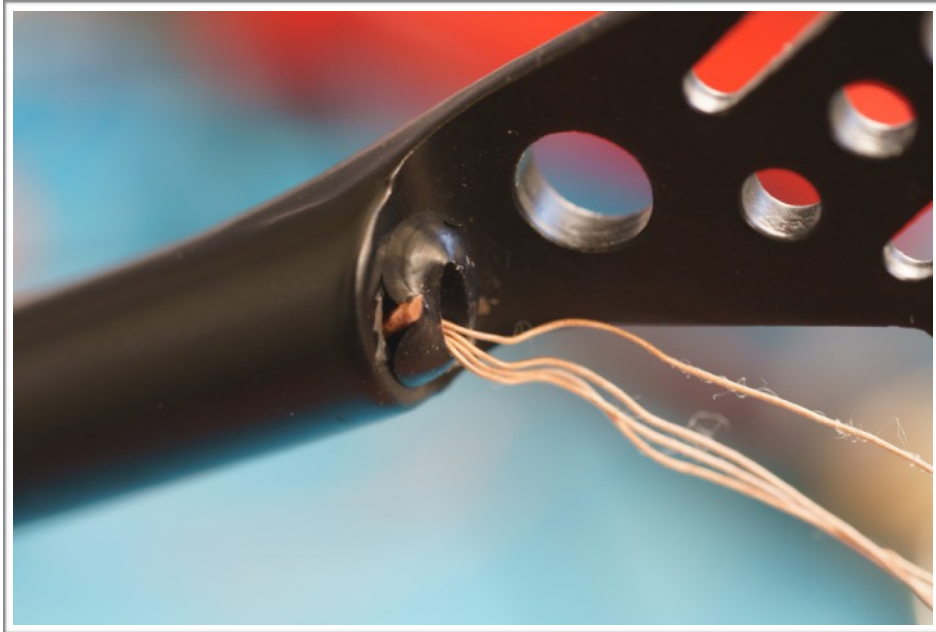
Fig 2 - head shell grommet in place with grounding rod
